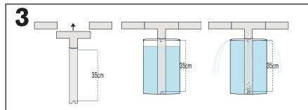
A condensation collector then needs to be attached. A condensation collector can be made from an old bottle or container. It must be tall enough to have at least 35cm between the bottom of it and the top where some holes must be put in to make sure the water doesn't overflow.
