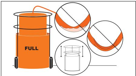
If the tank is full of gas, check the pipe system between the gasometer and the kitchen. Make sure always to run the pipeline with an inclination or else water will be stored. Check no pipes are broken or pinched. Make sure the inner tank can move up and down easily
