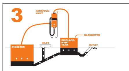
After approximately four hours the pressure reaches a high level and starts to push out a small portion of the material through the outlet. This material works very well as fertilizer on the fields. The system is designed to push about 20 percent of the organic material from the reactor up to the displacement tank.
