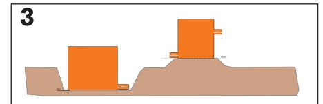
Make sure the spaces for the tanks are level and clean, then place the digester and the displacement tank in their right positions, making sure again they are the correct height apart.
