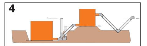
Connect the 6 pipes and the inlet, starting from the digester and working toward the displacement tank and outlet.
