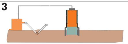
Place the upper tank inside the lower tank and attach the metal casing. Also attach the support poles to the casing and secure in the ground. FIll in the remaining space around the lower tank with earth to secure it, and level the ground around it.
