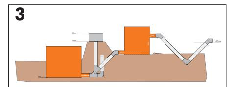
An inlet pit then needs to be created, this will make it easier and cleaner to deposit the organic waste into the system.
