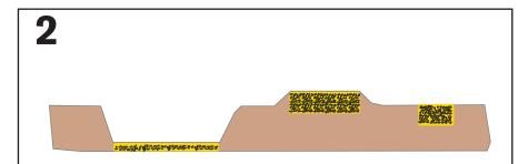
Mark out where the digester and displacement tank will be placed and level the area.
