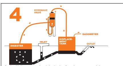
At the high pressure level the hydraulic valve opens and the gas escapes from the digester to the displacement tank. Because of this all the material that has been moved up to the displacement tank will move back to the digester. This stirs the organic material and the old material mixes with the new input. This cycle happens 6-7 times a day so that it is possible to make 2-3 times more gas than in traditional systems.
