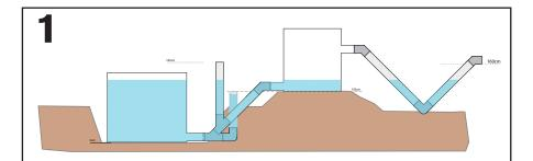
Once the pipes and tanks are connected, check for any leaks in the system by filling it with water through the inlet. There must be enough water to immerse all the piping joints which will be underground.
