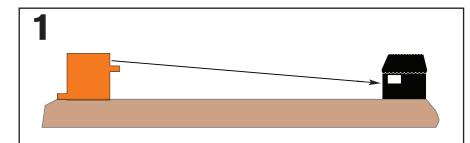
To connect the system, first decide on exactly where it is you want the gas to be supplied. From this point measure the distance to the gasometer to give an idea of how much piping you will need.
