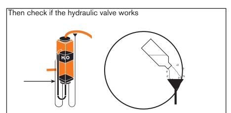
Make sure there is water in the system by observing if water from the lower can surges up to the upper can - if not, fill water in the funnel. You can never fill too much water in the hydraulic valve. Then observe it for a few hours and make sure the process is in function. This can be seen by that the levels of the water in the pipes and the containers changing, eventually also the water blown out from the u-tube.
