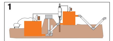
Connect the compressor to the digester, this will be used to test the pressure within the system and check for any leaks or breakages that may occur. Attach the big and small manometers to the connectors on the tanks. The big manometer should be connected to the digester and the small one should be on the displacement tank.
