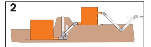
When you are sure the tanks and pipes are all water tight you can begin to cover the system, leaving the water in it. It is especially important to check the components which will be underground for any leaks or stresses to make sure you don't have to dig them up again. Fill in all the space around the digester with earth, leaving only the top half of it out of the ground, cover the piping joint on the outlet to make sure it is stable.
