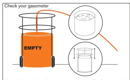
If the tank is at a low level it means there is no gas in it. Check the water level in the lower tank - fill it up if needed. Make sure the inner tank can move up and down easily.
