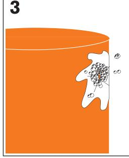
Whilst the pressure is maintained at 70cm in the digester, thoroughly check all surfaces for leaks or stresses. Leaks can be checked for by using water with soap in. Test the tanks and pipes by applying the water over them, if soap bubbles appear then it means there is a leak. These bubbles can be very small so attention is needed. Leaks should be checked for throughout the course of the testing, and any leaks found should be fixed as quickly as possible.
