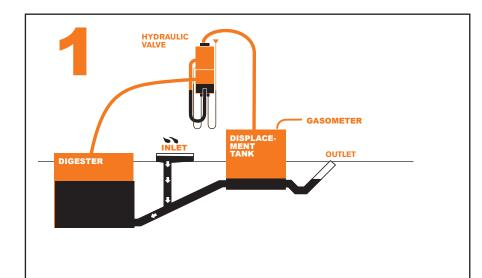
Organic material such as cow dung is deposited in the biogas systems inlet once or twice a day.
