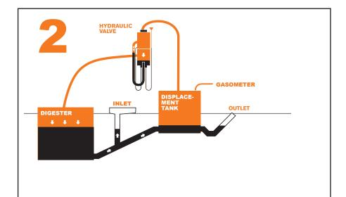
The biogas production builds up pressure inside the digester and forces a portion of the organic material up to the displacement tank.
